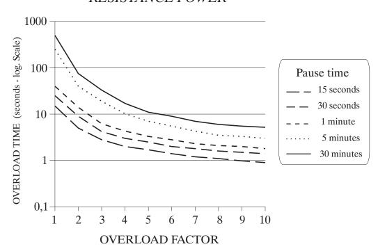
To calculate the value of the costant power (or rated) of the braking resistor using this graphic, it will be possible to apply the following formula:
